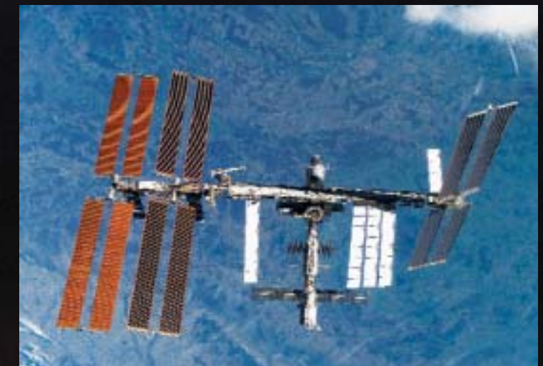
Backdropped by a colorful Earth, the International Space Station is seen from Discovery as the two separate. A station robot arm is visible as a white spar at the left end of the “track” that allows it to move from one end of the truss to the other. The damaged solar wing was at the extreme range of the arm's reach. The repaired site is the far lower array—about 40 percent of the way out toward the end where several “stitches” are visible as white lines that parallel the extended wing.
