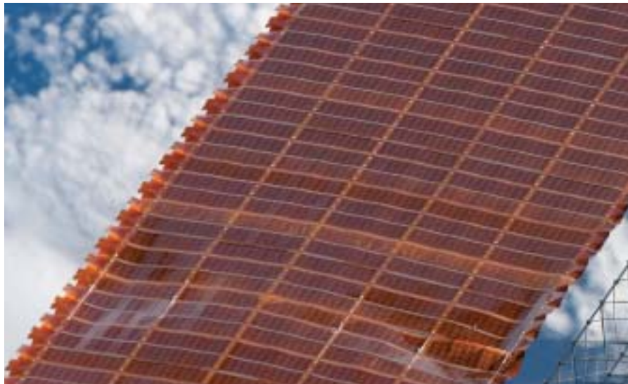
The repaired solar array was photographed by an STS-120 crew member aboard the space shuttle Discovery as it moved away from the International Space Station. The repair is in the foreground.
