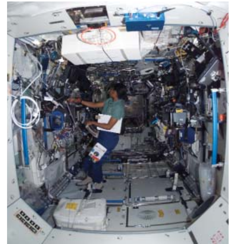
Astronaut Stephanie Wilson, STS-120 mission specialist, works the controls of the Space Station Remote Manipulator System (SSRMS), or Canadarm-2, in the Destiny laboratory of the ISS during flight-day-12 activities while the space shuttle Discovery is docked with the station.
