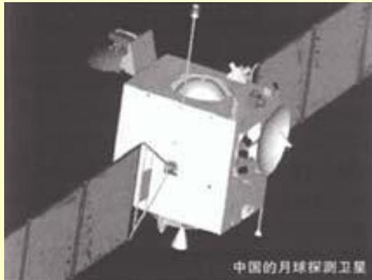
Lunar orbital probe (left) is to be built on basis of DFH-3 communications satellite (lower left)
