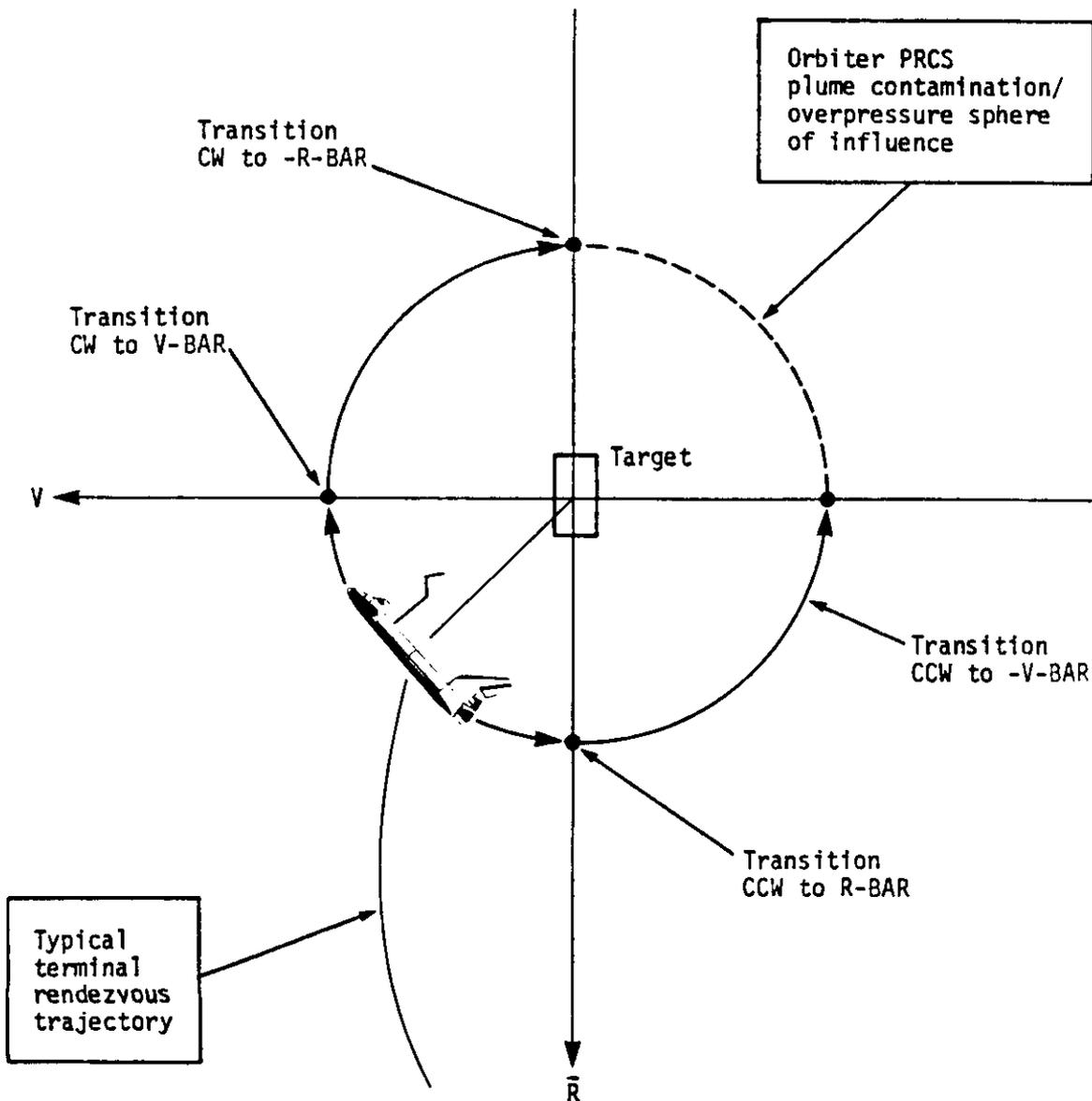
Figure 5-4.- Transition geometry.
