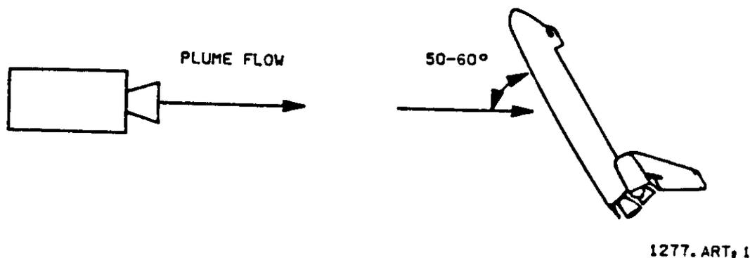
Figure 5-29.- Orbiter window protection attitude at SRM ignition.
