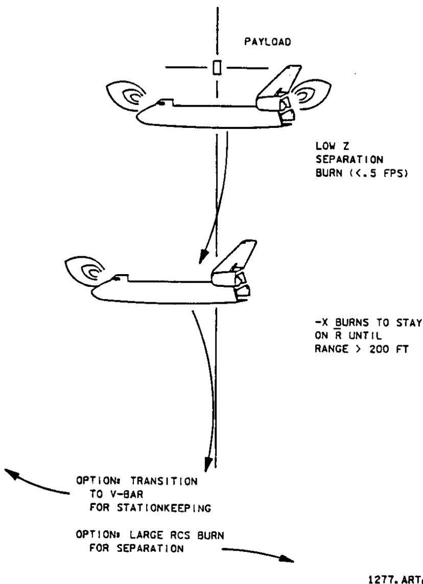
Figure 5-31.- Orbiter separation following RMS deploy (PL-centered LVLH frame of reference).
