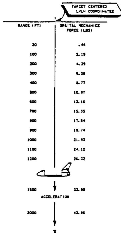
Figure 5-15.- Orbital mechanics forces during an R-BAR approach.
