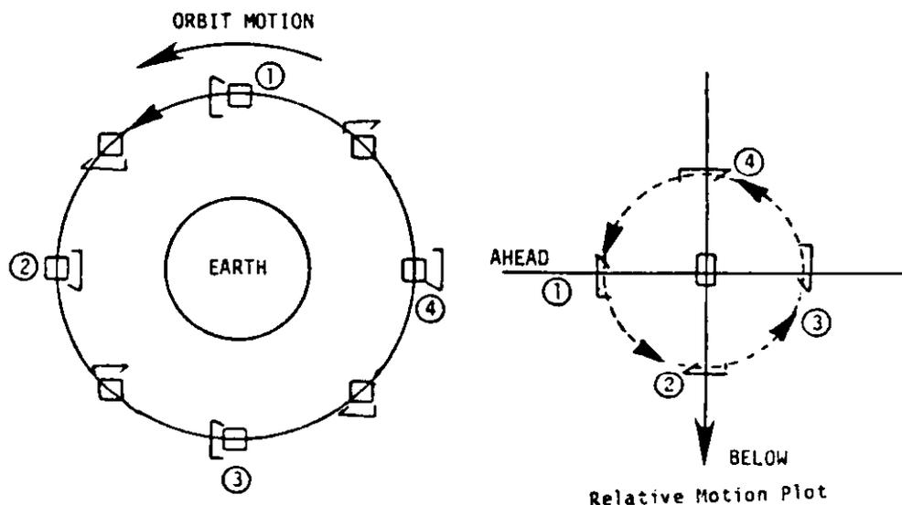
Figure 5-6.- Counterclockwise flyaround.
