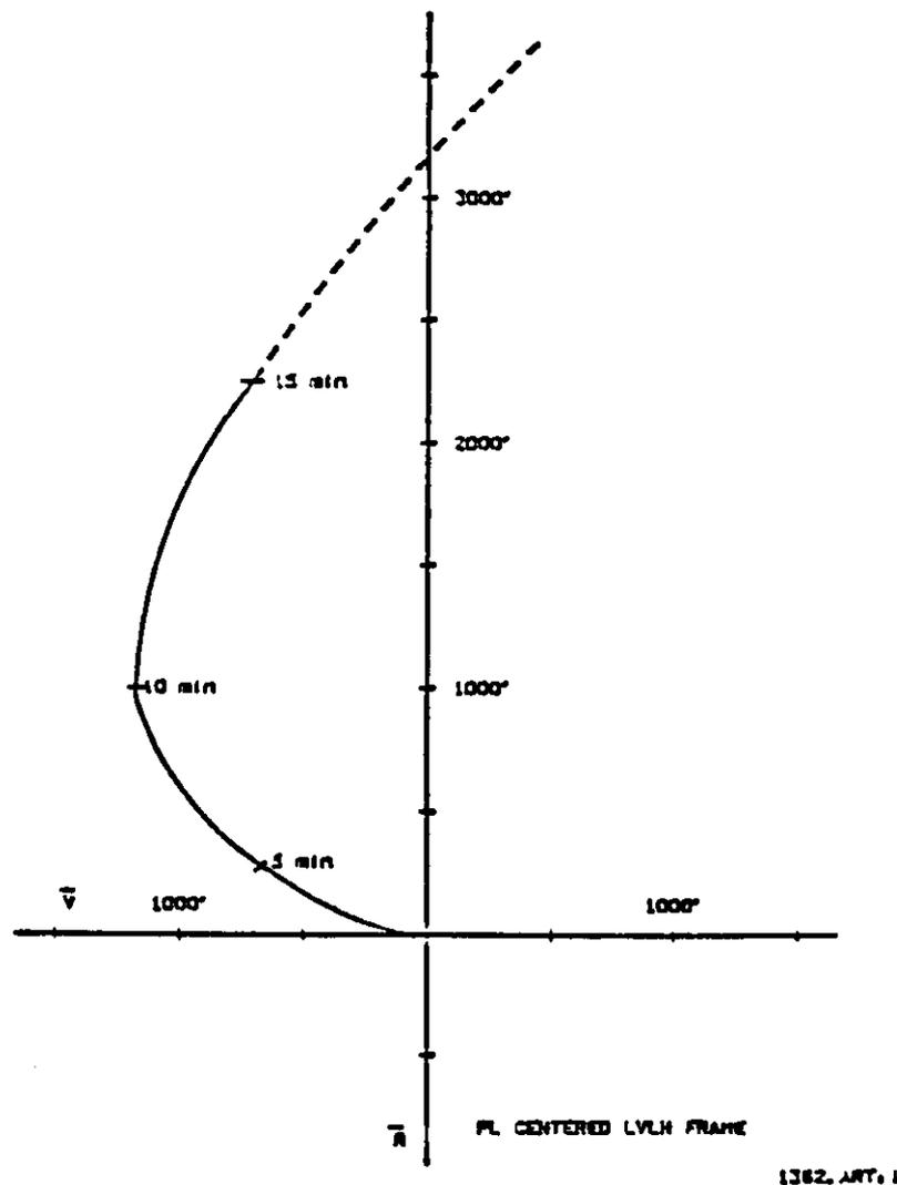
Figure 5-25.- Orbiter/PAM-D separation trajectory
