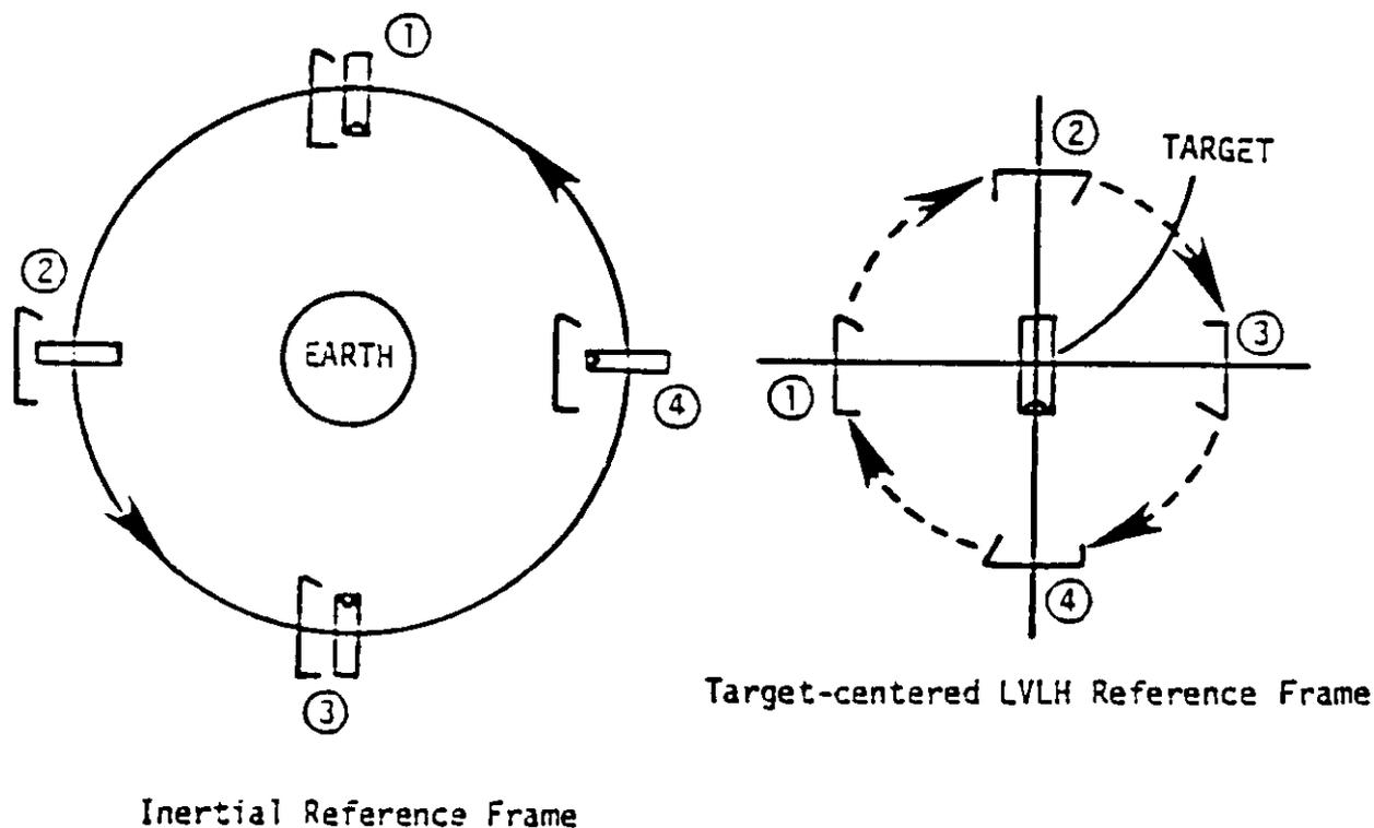
Figure 5-5.- Flyaround of an LVLH attitude hold TGT.
