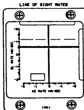
Figure 5-10.- Angle rates versus V-BAR stability
