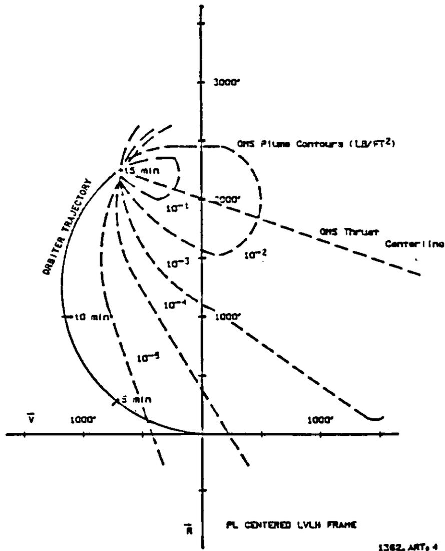
Figure 5-26.- OMS plume on PAM-D at SEP burn initiate.
