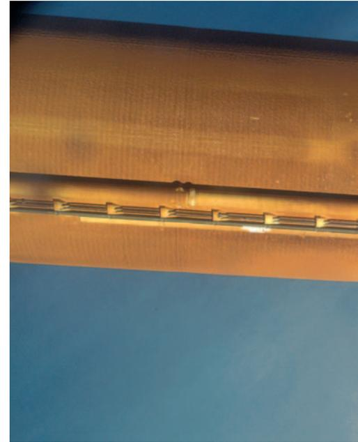
**RETURN TO FRIGHT: GAPS IN THE INSULATION FOAM ON DISCOVERY'S EXTERNAL TANK SHOW FOAM LOSS FROM THE TANK'S PROTUBERANCE AIR LOAD (PAL) RAMP. A FOAM IMPACT LED TO THE DESTRUCTION OF THE COLUMBIA SHUTTLE DURING RE-ENTRY ON FEBRUARY 1, 2003.**
