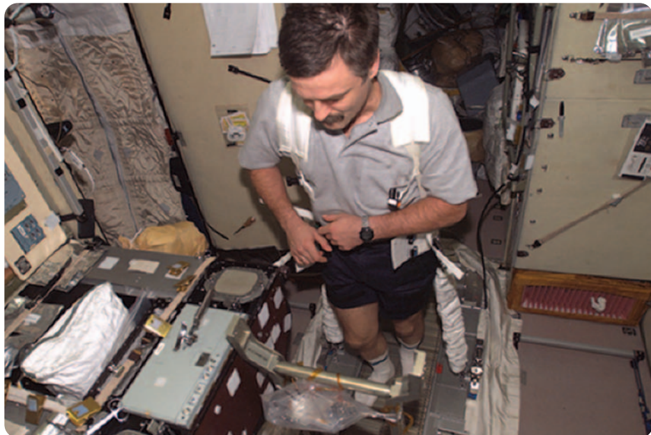
MR. FIX-IT: COSMONAUT ALEXANDER Y. KALERI, EXPEDITION 8 FLIGHT ENGINEER, PERFORMS IN-FLIGHT MAINTENANCE (IFM) ON THE TREADMILL VIBRATION ISOLATION SYSTEM (TVIS) IN THE ZVEZDA SERVICE MODULE ON THE INTERNATIONAL SPACE STATION (ISS). Image Credit: NASA
