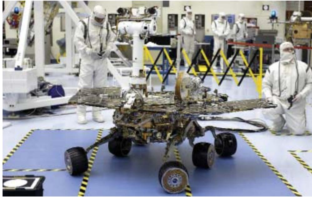
The Mars Exploration Rover has six wheels, each with its own individual motor. The two front and two rear wheels also have individual steering motors (1 each). These Rovers can turn a full 360 degrees, in place, and swerve and curve while driving.
